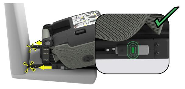
Place the car seat onto the vehicle seat and attach the ISOFIX connectors (H) to the ISOFIX attachment points in the vehicle. Confirm that the indicators (I) on both ISOFIX connectors has turned green.
