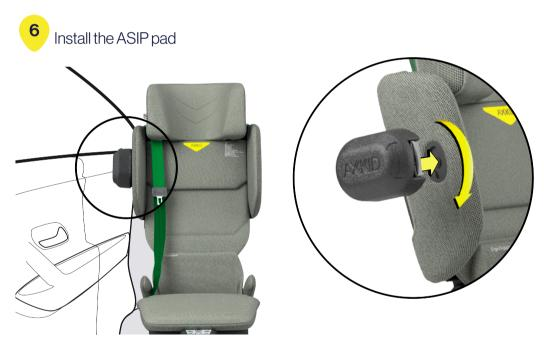
Install the ASIP pad (N) on the side of the car seat closest to the vehicle door. Align the ASIP pad attachment with the ASIP holder and attach it by pushing and rotating it into place.
