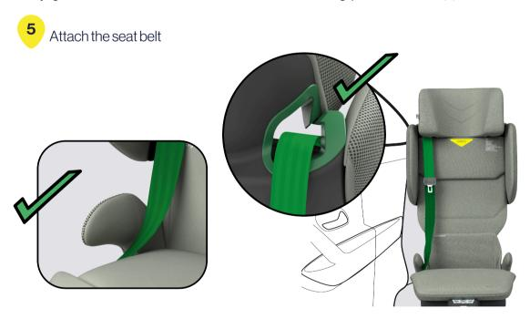
Pull out the vehicle seat belt and route the shoulder belt through the upper belt guide (M) and the lap belt under the lower belt guide (Q).
