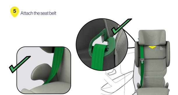
Pull out the vehicle seat belt and route the shoulder belt through the upper belt guide (M) and the lap belt under the lower belt guide (Q).
