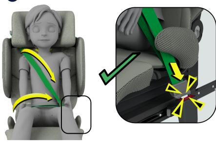
Seat the child in the car seat and extend the seat belt. After passing the seat belt over the child, both the lap-and shoulder belt must be routed under the lower belt guide (Q) on the opposite lower side of the car seat. Connect the vehicle seat belt to the belt buckle.
